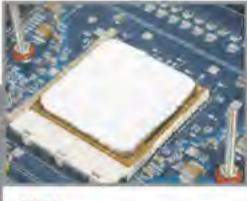
Note: Too much compound will decrease the performance of the CPU fan. The thickness should be between 1mm to 2mm.
